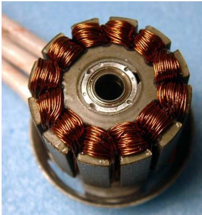
The stator is wound with several wires in parallel (commonly employed in commercial motors due to technological considerations) using a so called “distributed LRK” scheme.
