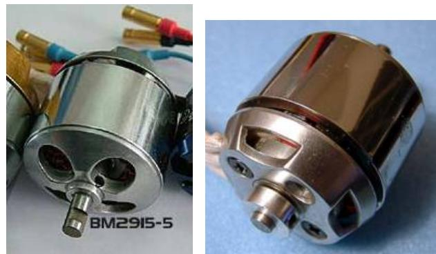
The motor mounts to the airframe via the rear flange on its stator. The rotating bell has 14 rare-earth magnets glued inside. The front of the bell has four cooling holes:
