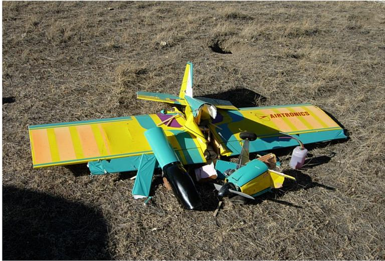
This is what can happen on take off when you don't do a preflight check and have the ailerons wires crossed.
