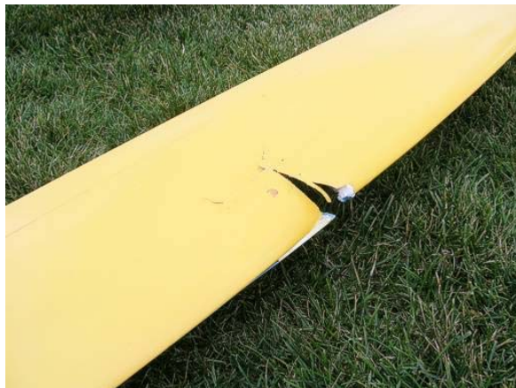
Result of a midair—the bang was heard from a mile away but the glider was still flyable
